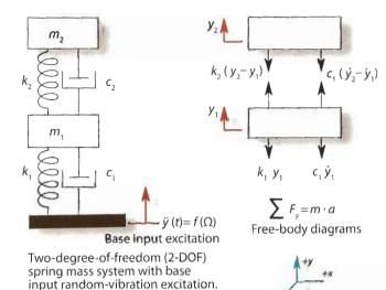
In this simple 2-DOF spring-mass system, m, and m, represent the individual concentrated mass -- units are lb-sec2/in.; k, and k, represent the spring rate or stiffness — units are lb/in.; c, and c, represent the damping — units are lb-sec/ in.; and y (t) and y (t) represent the displacement of each mass, m, and m, as a function of time — units are in inches.
